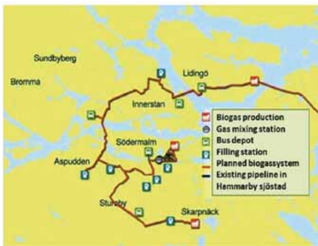
An overview of the future pipeline distribution system in Stockholm, indicating production plants, bus depots and filling stations.
